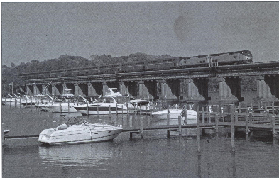
ABOVE: REBUILT P40s ON AUTO TRAIN — Amtrak has assigned six recently rebuilt General Electric P40s to its popular Auto Train. The six P40s, Nos. 814, 818, 830, 831, 832 and 835, were rebuilt with funding through the American Recovery and Reinvestment Act of 2009. A total of 15 P40s have been rebuilt for long distance service, which encompassed overhaul or replacement of all main components, including auxiliary generator power contactors, voltage regulator, batteries, trucks and air brake systems. This work was done at Amtrak's Beech Grove, Indiana, shop. Amtrak purchased 44 P40s from GE in 1993; after being in mainline service for a decade and a half they were removed from service and stored. Each Auto Train is now powered by a pair of the P40s, two others are kept at their facility at Sanford, FL. The southbound Auto Train with rebuilt P40s 835 and 832 is shown crossing Aquia Creek at Hope Springs Marina on April 16, 2012. This location is on the CSX RF&P Sub. near Stafford, VA. Digital photo/ Alex Mayes
